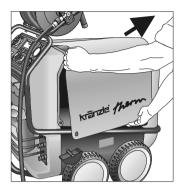
Open the right cover of the machine (without chimney)
