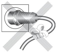
Do not damage the power cable or repair it incorrectly!
