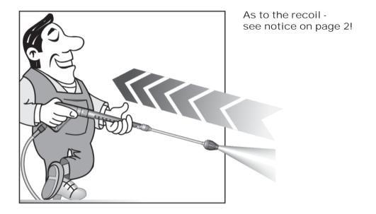
Apply the safety catch on the spray gun after each use, in order to prevent unintentional spraying!
