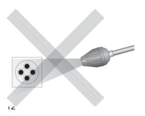
Never direct the water jet at a power socket!
