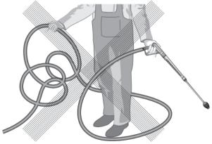
Never pull the high pressure hose if it has formed kinks or "nooses"! Never pull the hose over sharp edges!
