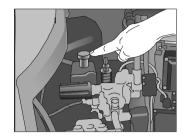
and check the oil level of the high pressure pump.
